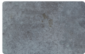
OXCP (Oxidized Copper) Oxidizers and heat are applied simultaneously to a natural copper surface, accelerating the development of protective verdigris in a range of green and white tones.
