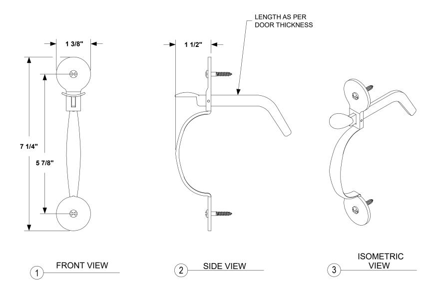
NOTE: Items are hand made one at a time. There may be slight variations in measurement and tolerances when comparing to actual Cad drawing.
